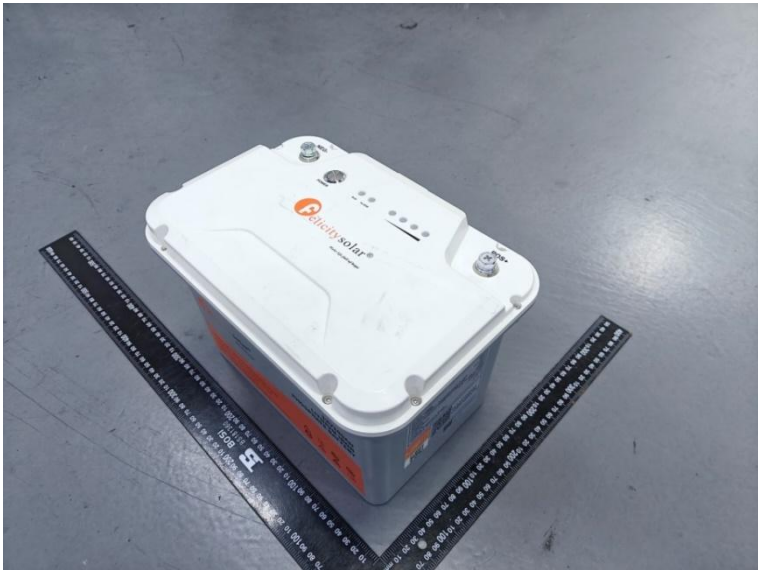
Battery: FLA12100PG2, 12.8V, 100Ah, 1.28kWh
